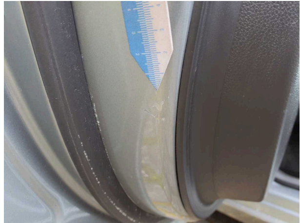
Beschädigung 6: Tür vorn links: Tür - Kratzer - Smart Repair
